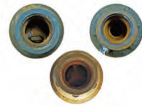
Inlet and outlet of worn pressure regulators.
