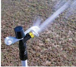
The diffuser distributes some of the flow closer to the sprinkler for better uniformity of application.
